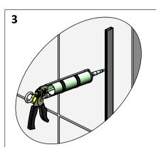
RUN A SMALL BEAD OF SILICONE DOWN THE INSIDE OF THE WALL PROFILES BEFORE FITTING GLASS. NOW SLIDE THE GLASS PANELS (ITEM 2) INTO THE PROFILES.
