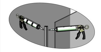
TO FIX THE OPTIONAL RETURN GLASS PANEL, FIRSTLY RUN A SMALL BEAD OF SILICONE DOWN THE INSIDE OF EACH GLASS SLOT IN THE CORNER PROFILE (ITEM 15) STOPPING 5mm SHORT AT EITHER END.
