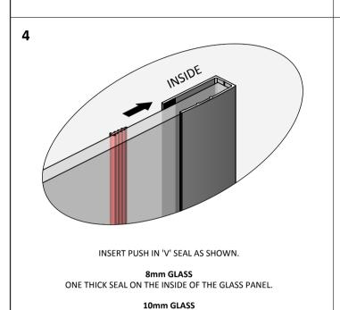
ONE THIN SEAL ON THE INSIDE OF THE GLASS PANEL.
