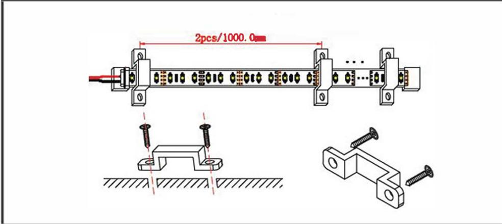
Using the rubber clips and screws that are supplied with this flexible strip, fix the strip to the desired location, as shown in the diagram above. Then connect the strip to the 15W IP44 rated driver (SE40560). Further instructions for the 15W IP44 rated driver are included in the driver pack.
