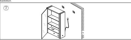
Keep the power off and connect the wires of the mirror to the wires exposed on wall. Hang the mirror cabinet to the wall brackets.
