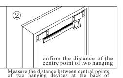
At the position 2 cm (3) below the central poin Mark the central point on the wall
