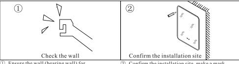
1. Ensure the wall (bearing wall) for installation could afford the weight of mirror.
