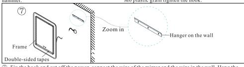
7. Fix the hook and cut off the power, connect the wire of the mirror and the wire in the wall. Hang the mirror on the hook directly. Rip the double-sided tapes back of mirror apart according to the actual
