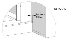
OFFER THE FRAME ONTO THE TRAY FIRST. ENSURE WALL PROFILES WILL REACH BOTH WALLS.
