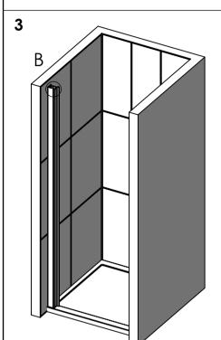
CHOOSE WHICH SIDE YOU WANT THE DOOR TO HINGE FROM AND THEN SLIDE THE MAGNET POST (ITEM 3) INTO THE OPPOSITE WALL CHANNEL. (DETAIL 'B')
