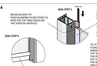
FIT THE DOOR BOTTOM SEAL (ITEM 18). IT SHOULD BUTT UPTO THE VERTICAL PROFILE WITH THE HINGES ON.
