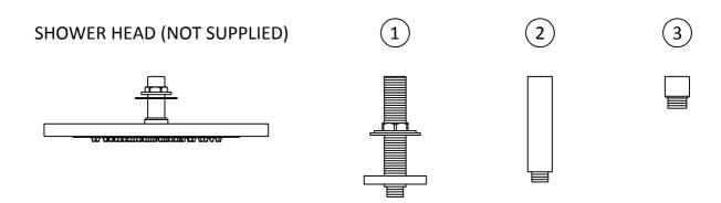
CONNECT YOUR PIPE WORK TO THE ARM USING THE 3/4" TAP CONNECTOR
