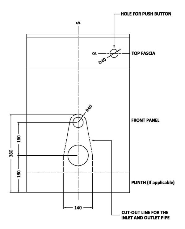
MARK OUT THE OPENING ON THE FRONT PANEL FOR THE INLET AND OUTLETS OF THE W.C. PAN. FOLLOWING THE ABOVE DIMENSIONS, CHECK THE SIZE AGAINST THE PAN BEFORE CUTTING OUT. DO NOT CUT OUT THE BOTTOM PLINTH!
