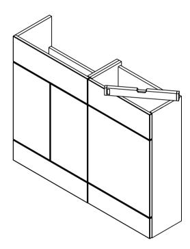
2. THE TOP FASCIA ON THE VANITY UNIT WILL NEED TO BE CUT-OUT TO RECEIVE THE BOWL OF THE BASIN. GENTLY REMOVE THE TOP FASCIA BY SLIDING UPWARDS TO RELEASE FROM THE FIXING BRACKETS.
