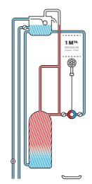
If you have a cold water tank in your loft and hot water cylinder (usually found in your airing cupboard) then you have a gravity fed system.
