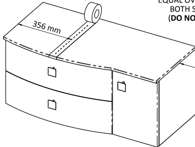
3. PLACE THE MARBLE ONTO THE UNIT WITH EQUAL OVERHANG BOTH SIDES. (DO NOT FIX)
