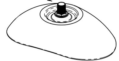
8. NOW REFIT AND SECURE THE MARBLE TOP USING SEVERAL SMALL BLOBS OF SILICONE ON THE UNIT TOP. ENSURE IT IS CENTRALISED.
