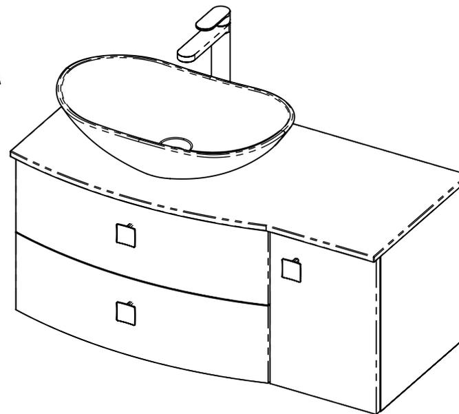
4. PLACE THE TAP AND BASIN IN THE DESIRED POSITION. THE BASIN WASTE CENTRE CAN BE **NO MORE THAN 270mm** FROM THE BACK EDGE
