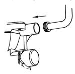
4. Insert the flush pipe and flush cone into the inlet hole on the Pan. Ensure the pipe is fitted securely into the Pan.
