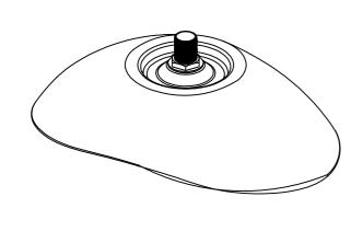
8. REFIT AND SECURE THE MARBLE TOP USING SMALL BLOBS OF SILICONE ON THE UNIT TOP EDGES. ENSURE THE TOP IS CENTRALISED. 9. FIT TAP AND BASIN. USE A SMALL AMOUNT OF SILCONE TO SECURE THE BASIN IF REQUIRED. ALLOW 24 HOURS FOR SILICONE TO FULLY DRY.
