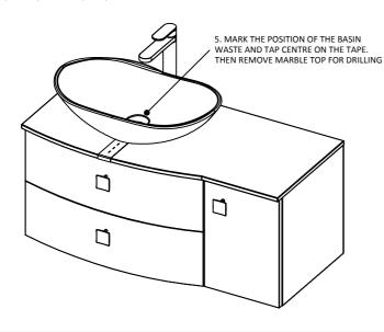
5. DRILL THE MARBLE Ø35mm FOR TAP AND Ø75mm FOR THE BASIN WASTE ON A SUPPORTED SURFACE. USE A DIAMOND CUTTER WITH COOLANT AS REQUIRED.
